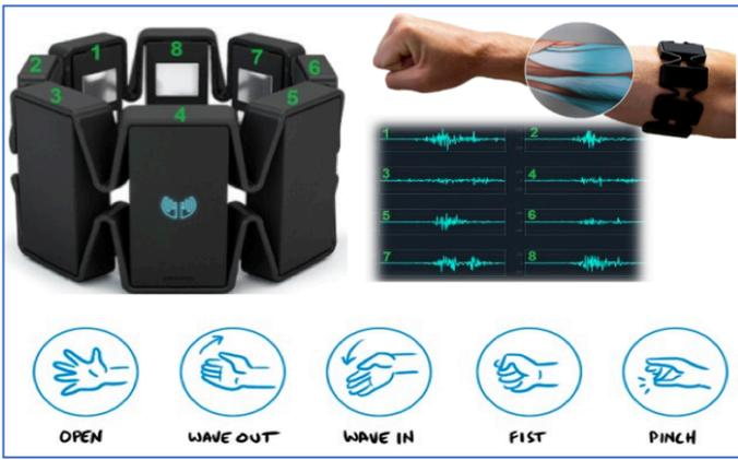
Fig. 6. Myo armband sensor by Thalmic labs. The bottom images present the possibilities for gestures recognition when using this sensor.
